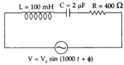
(ii) Without making any other change, find the value of the additional capacitor Cv to be connected in parallel with the capacitor C, in order to make the power factor of the circuit unity. (Delhi 2017)
