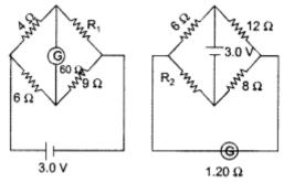
Figure shows two circuits each having a galvanometer and a battery of 3 V. When the galvanometers in each arrangment do not show any deflection, obtain the ratio  $R_1/R_2$ .
