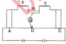
Find the position of the null point when the  $10 \Omega$  resistance is instead connected in series with resistance 'Y'. Determine the values of the resistances X and Y. (Delhi 2008)
