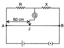
If the galvanometer and battery are interchanged, then there will be no effect on the position of balancing point.
