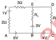
Question 65. Calculate the current drawn from the battery by the network of resistors shown in the figure. (Comptt. All India 2015)
