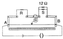
Question 80. In a meter bridge, the null point is found at a distance of 60.0 cm from A.
