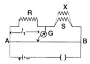
Question 78. Write the principle of working of a potentiometer. Describe briefly, with the help of a circuit diagram, how a potentiometer is used to determine the internal resistance of a given cell. (Delhi 2009)
