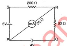
Question 44. The network PQRS, shown m the circuit diagram, has the batteries of 5 V and 10 V and negligible internal resistance. A milliammeter of  $50\Omega$  resistance is connected between P and R. Calculate the reading in the milliammeter. (Comptt. All India 2012)
