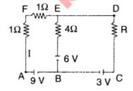
Question 92. Calculate the value of the resistance R in the circuit shown in the figure so that the current in the circuit is 0.2 A. What would be the potential difference between points B and E? (All India 2012)
