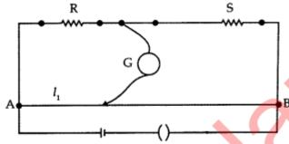
An unknown resistance X is now connected in parallel to the resistance S and the balance point is found at a distance  $l_2$ . Obtain a formula for X in terms of  $l_1$   $l_2$  and S. (Outside Delhi) R
