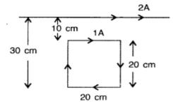
Calculate the magnitude and direction of the net force exerted on the loop due to the current carrying conductor. (Comptt. All India)
