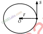
For example, an object moving in a circular path due to centripetal force acting on it. At any instant of time, a constant acceleration due to the centripetal force act on the object along the radius towards the centre while the direction of displacement is tangential to the circle. That is, force and displacement are perpendicular to each other and hence no work is being done.
